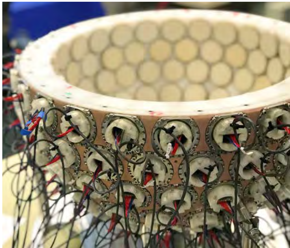
At the Karlsruhe Institute for Technology, researchers are developing a 3D ultrasound computer tomography instrument to use for radiation-free breast cancer screen. This measuring aperture (above) is outfitted with many individual ultrasound transducers. | Foto: KIT
